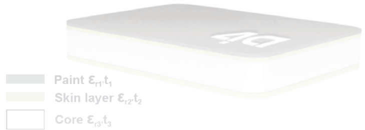
Figure 3: A-Radome configuration protected with specific coating.
